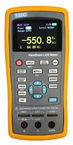
This meter will accurately measure capacitors, inductors and resistors using the test frequencies of 100Hz, 120Hz 1 kHz, 10kHz and 100kHz.
